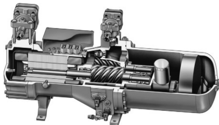
ပုံ ၁၄-၄၀ Semi-hermetic screw compressor with built-in oil separation
