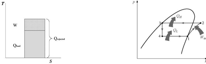
ပုံ ၇-၁ Carnot cycle for refrigeration
