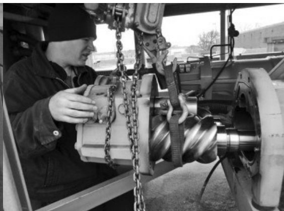
ပုံ ၂၁-၁၆ Rotary screw chiller overhaul
