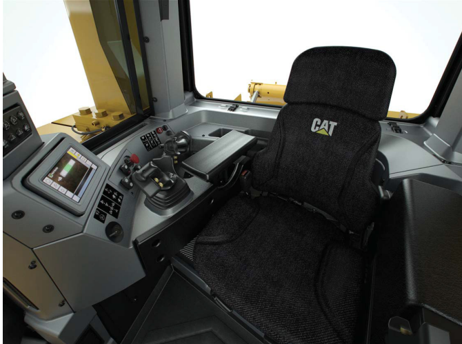
ç (5.8) Operator Station
