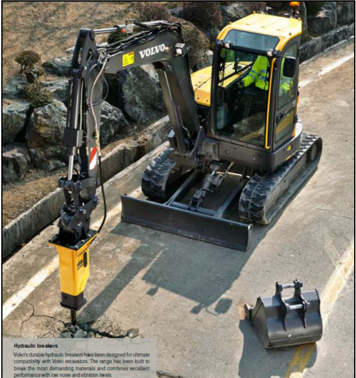
ပုံ (6.4) Volvo Excavator using with Hydraulic Breaker
