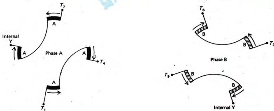
Fig (3-84) A circular diagram of a four-pole, two-voltage, short jumper, one- and two-wye motor.
