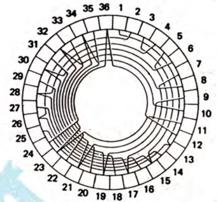
Fig (2-37) Cross connections of commutator bars for a six-pole motor having 36 bars, pitch 1 and 13.
