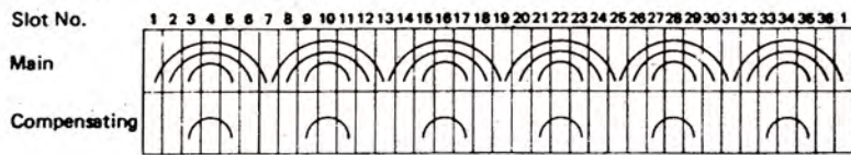
Fig (2-55) A layout of a six-pole compensated repulsion motor. Note the location of the compensating winding in relation to the main winding. The compensating winding is generally wound into the slots first.
