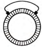
Fig (2-9) The assembly of the short-circuiting device of a brush-riding, repulsion-start, induction-run motor.
