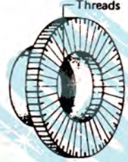
Fig (2-24) A radial commutator that is pressed on the armature shaft.
