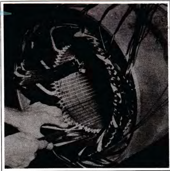
Fig (3-40) Winding and insulating a three-phase stator.
