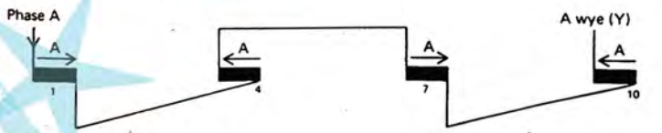
Fig (3-53) (a) Connections of groups of phase A.
