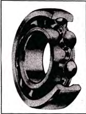
Fig (3-148) A ball-bearing illustration showing the components.
