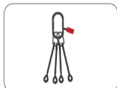
Figure 8: Use a master link with sub-links for all three- or four-legged wire rope slings.
