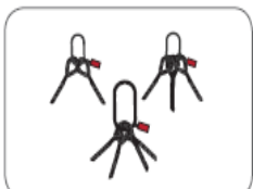
Figure 7: Use a single master link instead of placing wire rope slings directly on the load hook.
