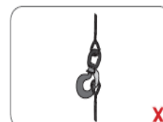
Figure 10: Sling fouled on latch.
