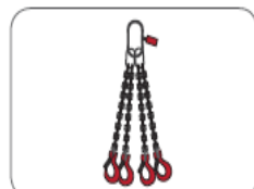
Figure 6: Use a master link with sub-links for three- or four-legged chain slings.
