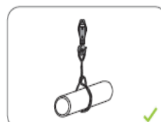
Figure 9: Prevent fouling of safety latch on load. Sling in base of hook.
