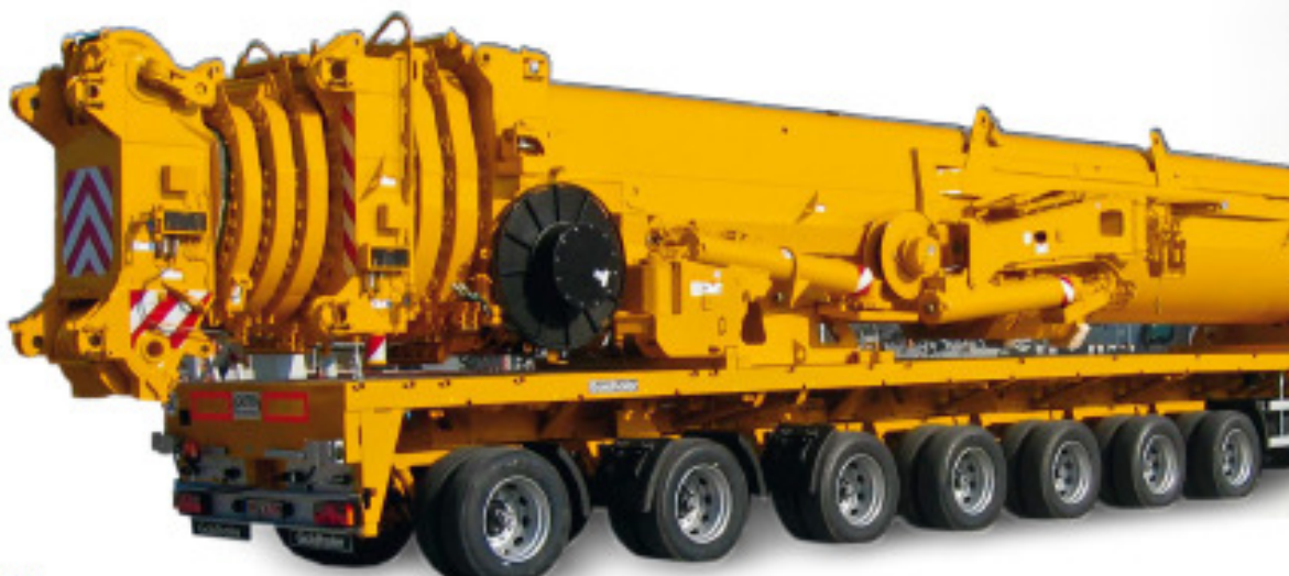
100 m telescopic boom + Y-suspension Stated weights: without boom lifting unit
