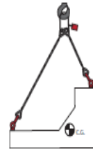
Figure 4: Good load control starts with rigging the load to the centre of gravity directly below the load hook.
