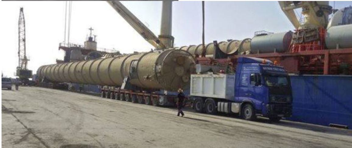
Record-breaking transport operation from Turkey to Arbil of a 247 ton refinery boiler 62 meters long
