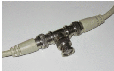
10BASE2 cable with BNC T-Connector
