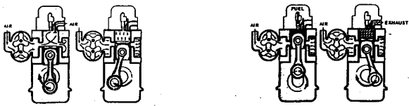
FIG. 1-7 IN GM'S Two cycle diesel engine: blower supplies air to cylinder through inlet ports. Hot compressed air fires fuel mixture. Fresh charge of air for next power cycle pushes exhaust gases out through open exhaust valves.
