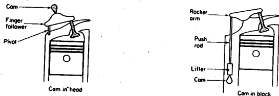
FIG. 1-17 Typical camshaft arrangement.
