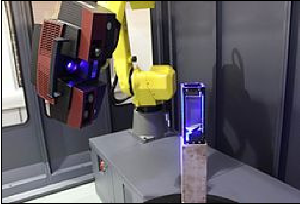
Robot scan using PowerINSPECT.
