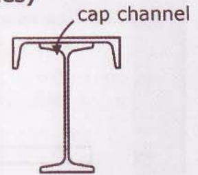
S12x3.18 with C10x15.3 cap channel
