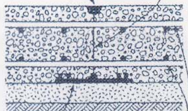
(b) Partial contraction joint in reservoir wall
