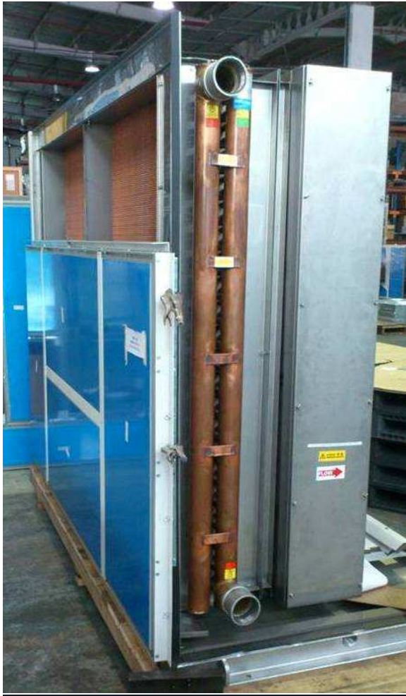
Figure 3. AHU Coil Section
