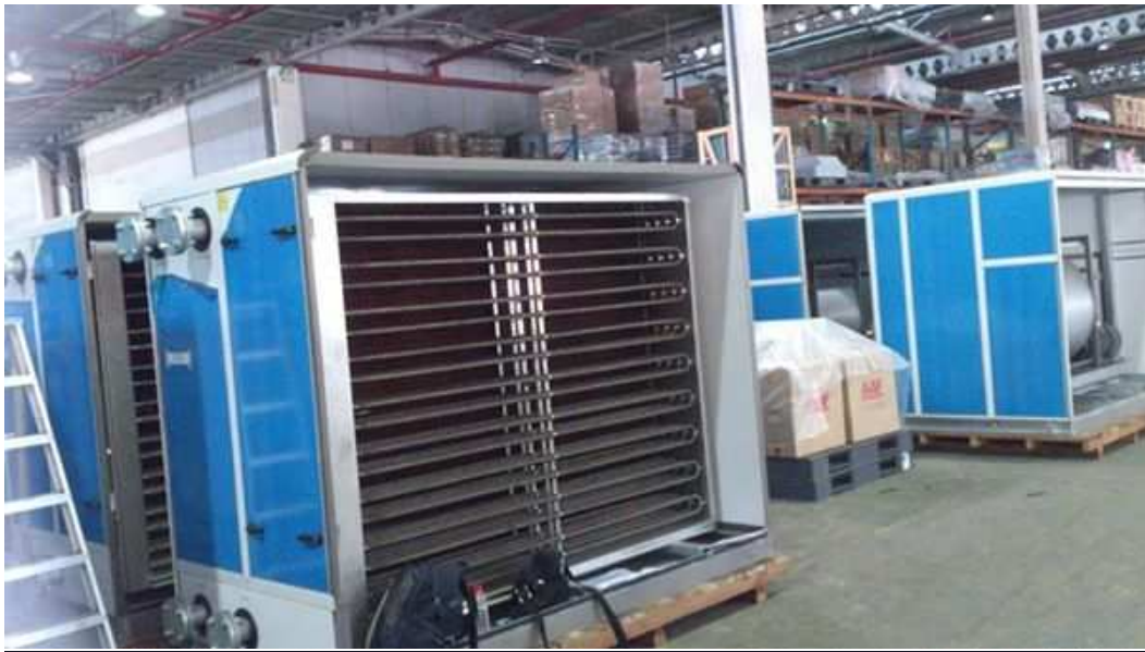
Figure 5. AHU Heating Coil
