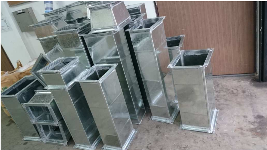
Figure 4. Rectangular ducts and fittings
