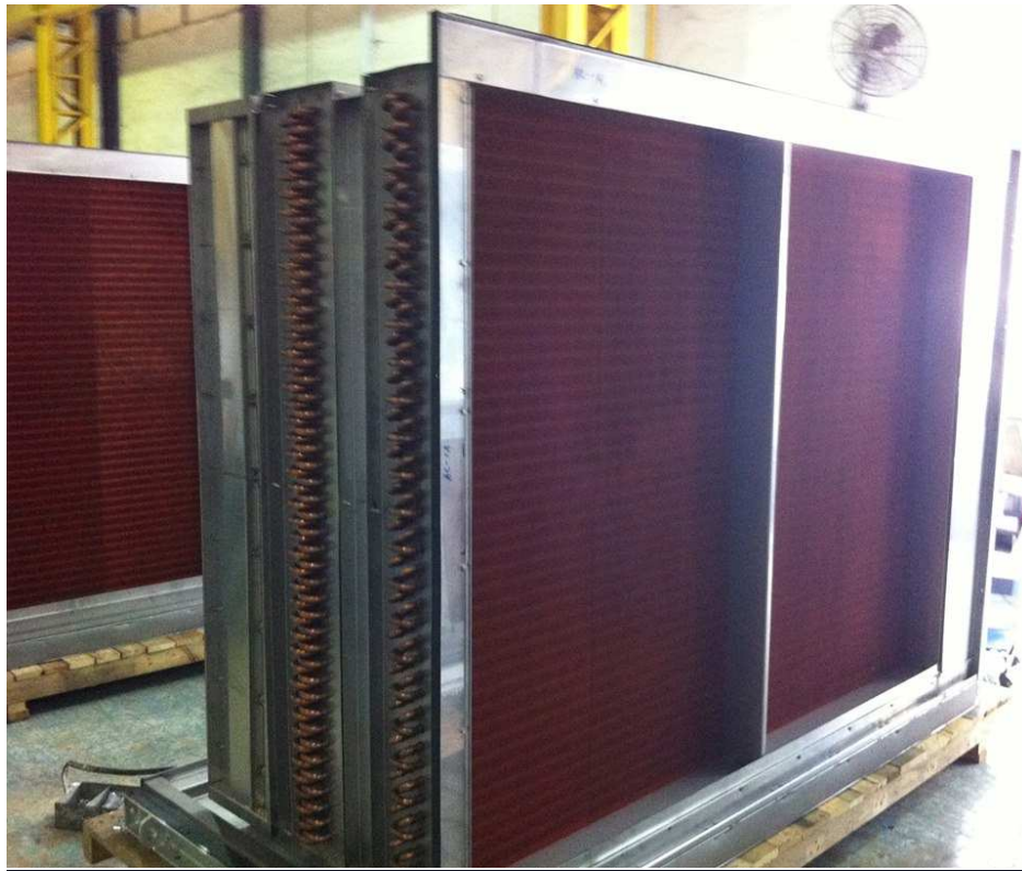
Figure 4. AHU Cooling Coil
