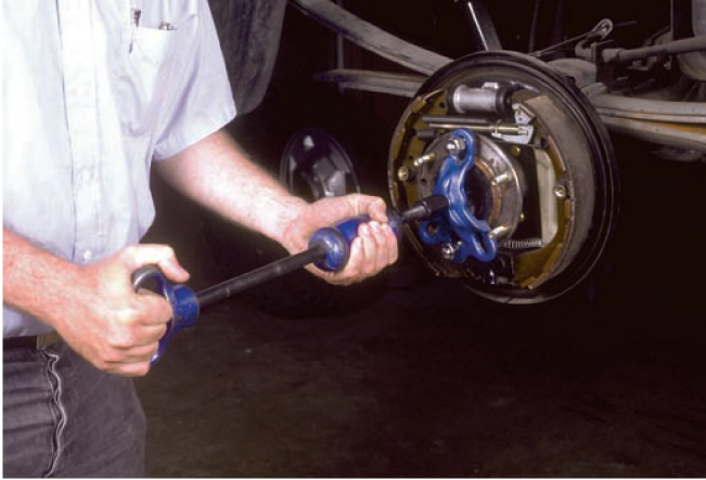
Fig (2-54) Using a slide hammer-type puller to remove a drive shaft.
