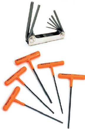
Fig (2-33) Top - A handy tool containing many different Allen wrenches. Bottom – Tee-handle Allen wrenches designed for better gripping and easier torque application.
