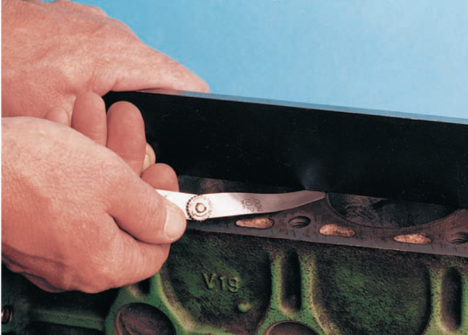
Fig (2-27) Using a feeler gauge and precision straightedge to check for warpage
