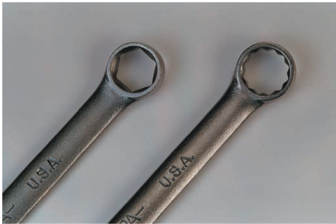
Fig (2-32) Six-point and twelve-point box-end wrenches are available
