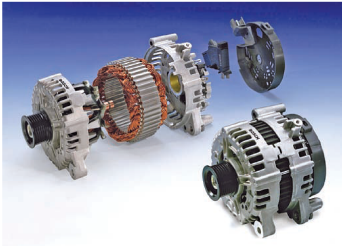
Figure (1-13) The major components of a late-model AC generator
