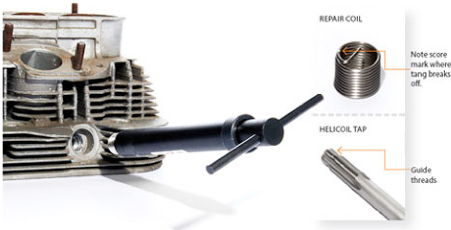
Fig (2-12A) Spark plug thread tap
