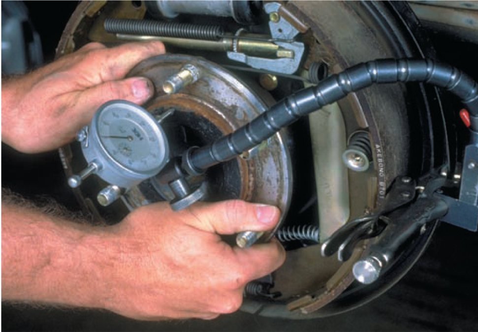
Fig (2-29) This dial indicator setup will measure the amount this axle can move in and out
