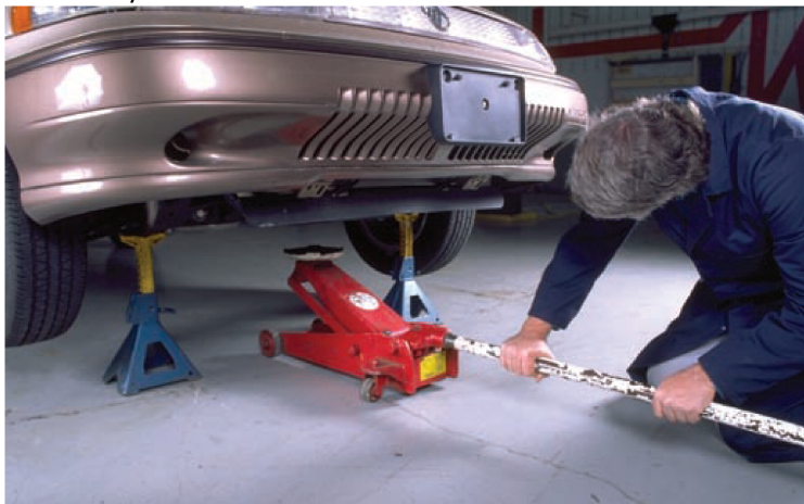
Fig (2-62) Whatever you have raised a vehicle with a floor jack, the vehicle should be supported with jack stands.
