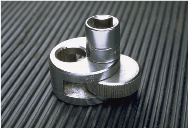
Fig (2-49) Stud installation / remove tool
