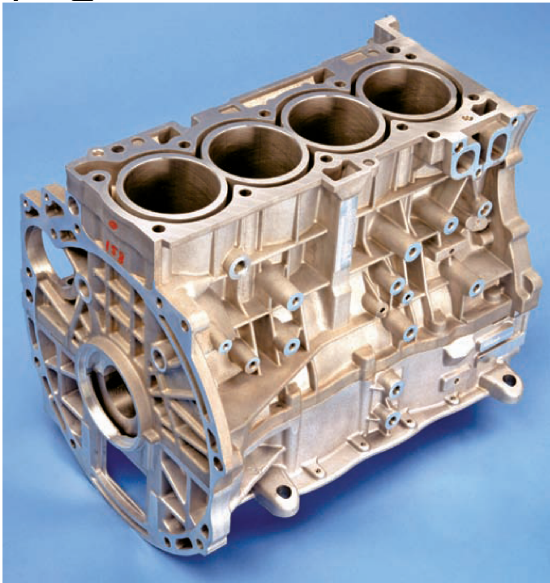
Figure (3-21) The cylinder block for an inline engine.
