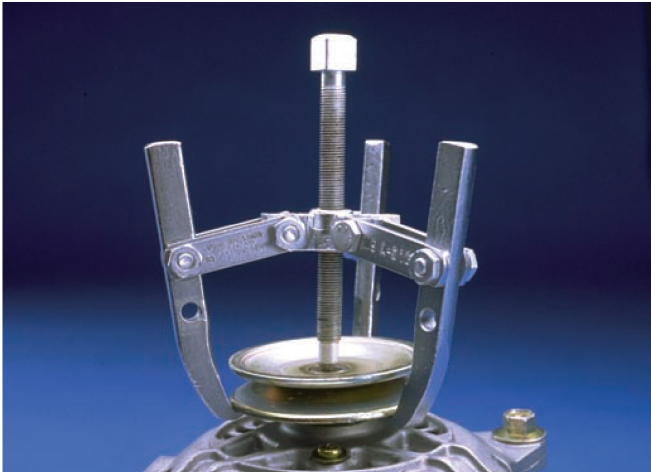
Fig (2-55) The jaws on this puller are reversible to allow for inside and outside pulls.
