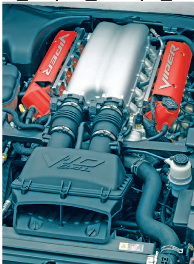
Figure (1-9) The intake system for a V-10 Engine
