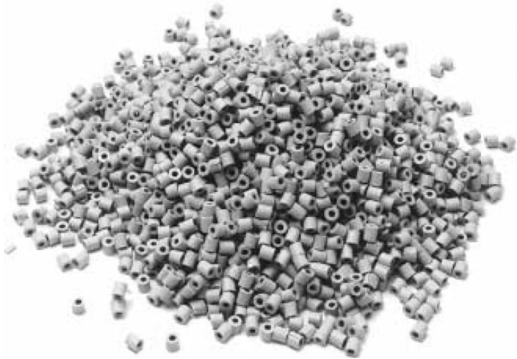
Packing material for column
