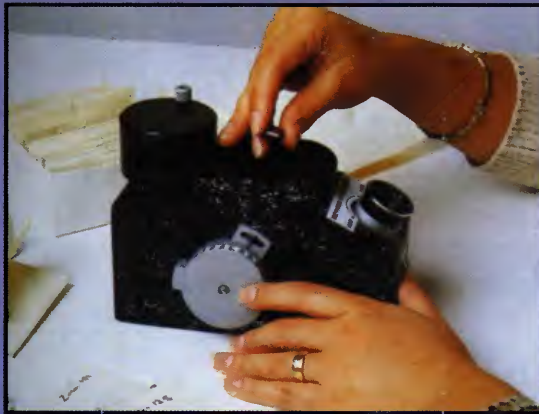
ပုံ (၁၁-၆) Placing a gem inside a Brewster Angle Meter.
