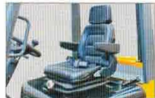
The optional of semi or full suspension seat with safety belt and arm rest.
