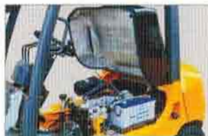
Engine cover with gas-filled cylinders and sound absorbing material.
