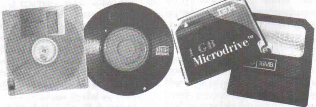
A 3.5-inch floppy (left), and an 8-cm CD-R (right). The CD-R holds over 120 times the amount of data held by the floppy.
