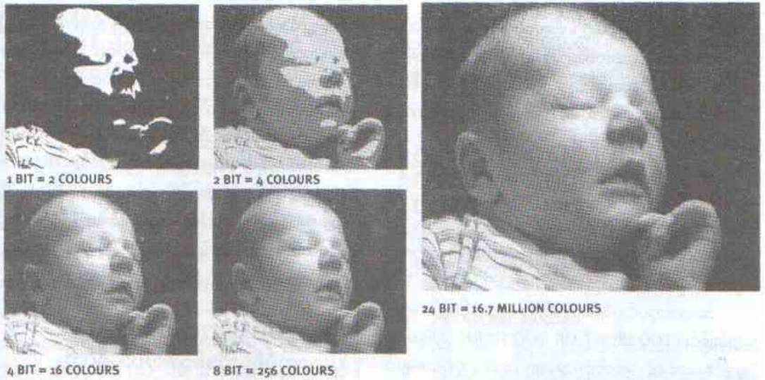
Fig 35 - The colour depth of a file determines the numbers of colours possible in the image.
