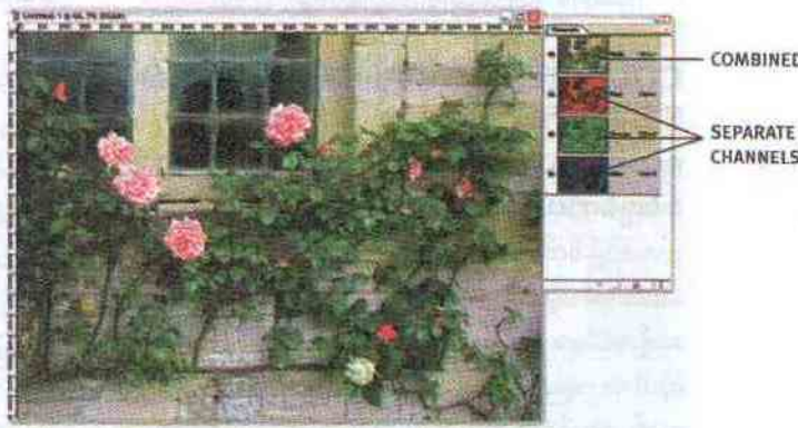
Fig 5 - Colour digital files are made up of red, green and blue channels which are stored separately and are then recombined when printed or viewed on screen.
