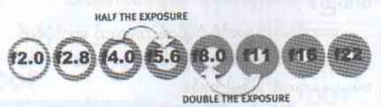
Fig 19 - The aperture series is organized in terms of F-stop numbers, each allowing half or double the amount of light into the camera than the one before.
